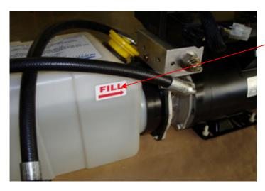
NOTE: Do not overfill. Fluid to this line when lift is in full upright position (as lift deck is lowered, fluid level will drop in tank, this is normal).
