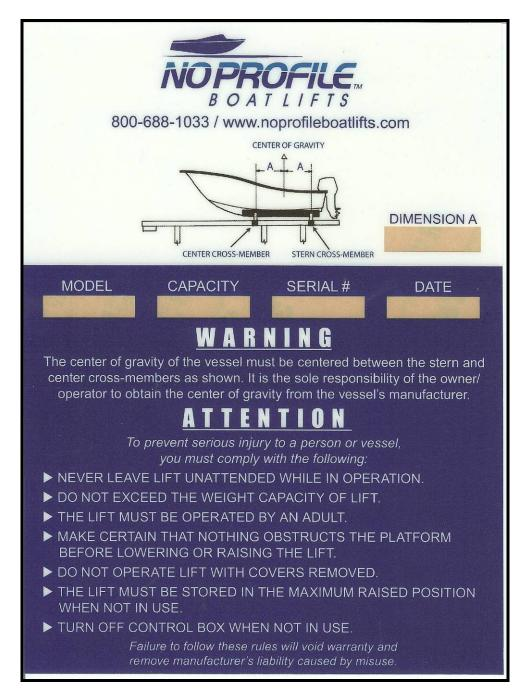
The No Profile Platform Lift is not intended to be used as an extension of a fixed dock. Limit personnel to occupants of vessel being launched or retrieved. No persons should be standing on deck, while Lift is in operation.
