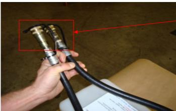
Hydraulic Quick-Disconnect (Left Hose – Lowers Lift) (Right Hose – Raises Lift)
